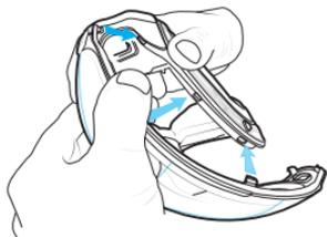
1. Start at one end of the goggle. Align teeth and assemble into goggle chassis. Caution: Use light pressure only when assembling the ends of the goggle into the chassis.
