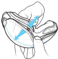
4. Pull lens away from frame near nose section. Avoid pulling on the face foam.
