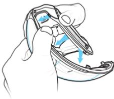
7. Carefully pull lens retention teeth away from frame.
